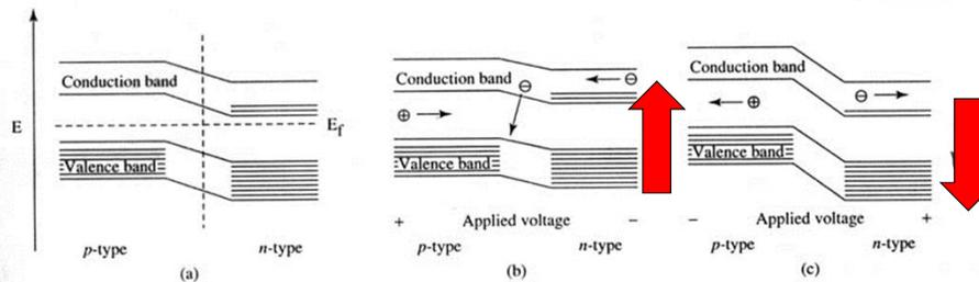
**FIGURE 7-15** Band-energy Diagram of a  $p$ - $n$  Junction. (a) At equilibrium, the two Fermi levels are at the same energy, changing from the pure  $n$ - or  $p$ -type Fermi levels because a few electrons can move across the boundary (vertical dashed line). (b) With forward bias. Current flows readily. (c) With reverse bias. Very little current flows.
