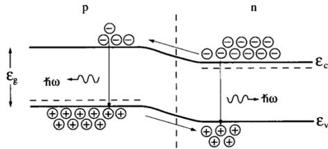
**Figure 5.1** Injection of minority carriers in a forward-biased p-n junction leading to spontaneous emission of photons.
