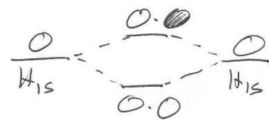
\* note, the resulting two orbitals are nearly identical in energy because of the large inter nuclear distance (poor overlap).
