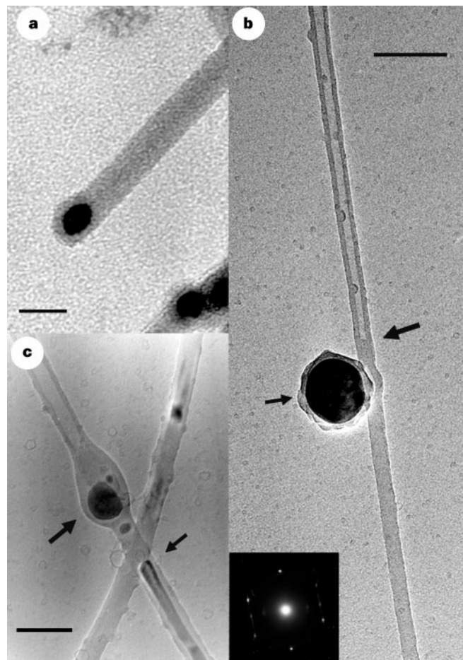
Figure 2 NT/SiNW junctions grown from SiNWs with a common Fe/Au catalyst. a , TEM image (EM420; Philips) of SiNW produced with a Fe 0.9 Au 0.1 catalyst. The 15-nm-diameter NW terminates in a Fe–Au nanocluster that appears as a dark, solid sphere. b, c , TEM images of NT/SiNW junctions. The hollow NTs are oriented at the top of both images and the solid SiNWs at the bottom. b , The large black arrow highlights the junction position. The small arrow indicates a metal catalyst cluster that was probably excluded from the junction during growth. The inset corresponds to an electron diffraction pattern recorded with the beam perpendicular to the NT/SiNW axis. The diffraction spots show that the SiNW maintains its crystalline structure after NT growth. c , The larger arrow highlights the junction region that contains a metal nanocluster. The contrast variation highlighted by the smaller arrow corresponds to SiNW (see the text for details). The scale bars in a, b and c are 20, 50 and 50 nm, respectively. Samples were prepared as follows. A pulsed Nd–YAG laser (532 nm, 7-ns pulse width; GCR-16S; Spectra-Physics) was used to ablate a Fe 0.9 Au 0.1 solid target placed within a growth system 8 . The ablation was performed for 10 min in 20-torr 10%/90% silane/He (99.998%; Matheson Gas Products), 20 standard cm 3 min -1 at 450 °C. NTs were grown from the SiNWs for 30 min in 300-torr ethylene (99.5%; Matheson Gas Products), 20 standard cm 3 min -1 at 600 °C.
