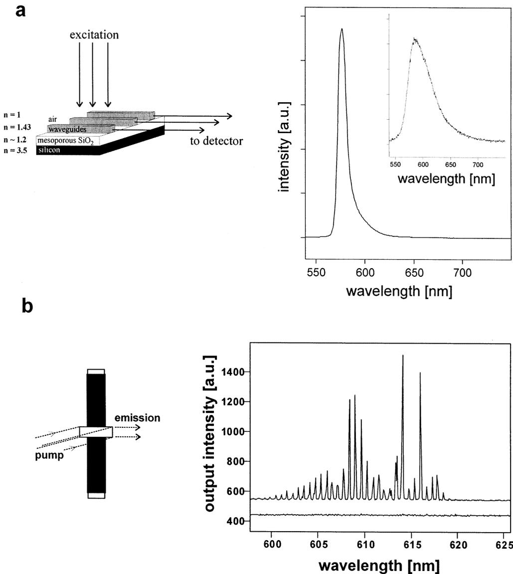
Fig. 5. (a) Amplified spontaneous emission in rhodamine 6G-doped mesostructured waveguides and (b) lasing in rhodamine 6G-doped  $\mu$ ring lasers. The pictures on the left depict the macroscopic structures and the pumping geometry, the spectra on the right show the emission below and above the threshold.
