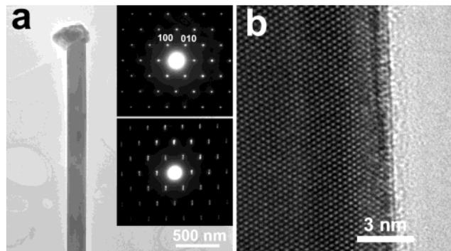
**Figure 2.** (a) TEM image of a GaN nanowire with an iron metal alloy droplet on its tip. Insets are electron diffraction patterns taken along the [001] zone axis. (b) Lattice-resolved TEM image of the nanowire.
