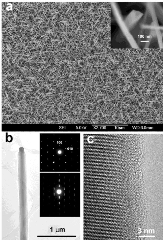
**Figure 1.** (a) FESEM image of the GaN nanowires grown on a gold-coated *c*-plane sapphire substrate. The inset shows a nanowire with its triangular cross section. (b) TEM image of a GaN nanowire with a gold metal alloy droplet on its tip. Insets are electron diffraction patterns taken along the [001] zone axis. The lower inset is the same electron diffraction pattern but purposely defocused to reveal the wire growth direction. (c) Lattice-resolved TEM image of the nanowire.
