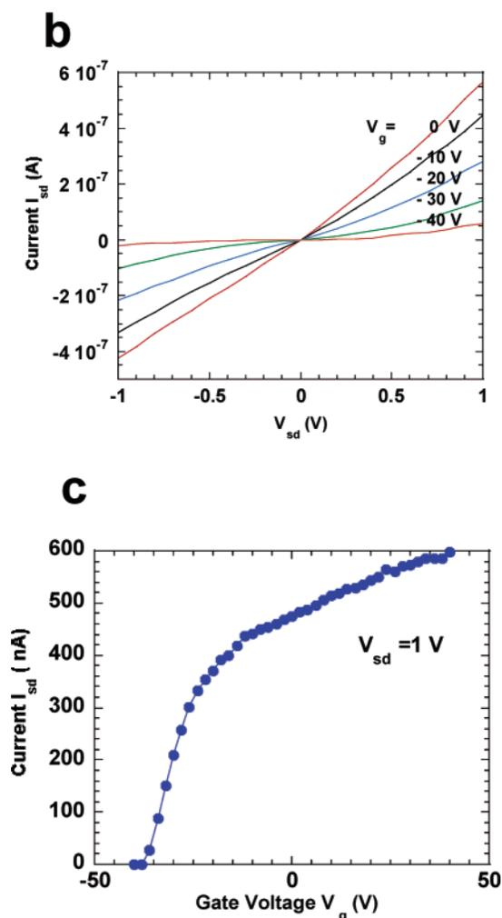
**Figure 5.** (a) SEM image of a GaN nanowire connected with two electrodes for the transport study. The inset is an illustration of the GaN transistor layout. (b) Current–voltage measurement at different gating voltages for the GaN nanowire. (c) Drain current as a function of the gate voltage ( $V_g$ ) for the GaN nanowire.
