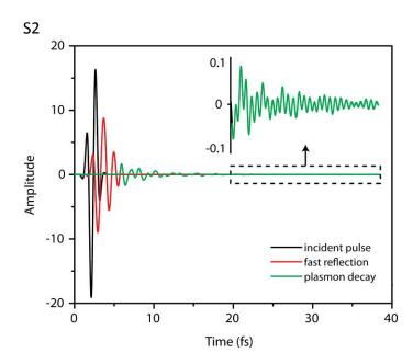
**S2**. Simulated electromagnetic response of a nanocrystal slab with 6-nm spacing. After subjecting the slab to an incident light pulse (black), light is either immediately reflected (red) or coupled into a slowly decaying plasmon resonance (green). Inset: The tail-end amplitude displayed for clarity.
