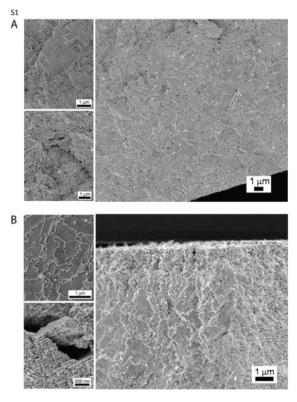
**S1**. Nanocrystal superlattices composed of different polyhedral building blocks. Assemblies of (A) cuboctahedra and (B) cubes were fabricated by drying a droplet of the appropriate colloidal suspension on a solid substrate. SEM images were obtained after cleaving the evaporated droplet.
