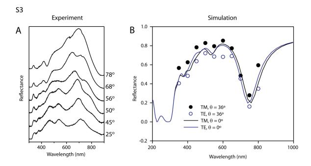
**S3**. Angular and polarization dependence of optical reflectance. (A) Reflectance spectra of a closest-packed supercrystal assembly taken at different angles of incidence. Spectra were obtained using fiber optic couplers for excitation and collection. (B) Simulated reflectance curves for an off-axis angle of incidence and rotated polarization.
