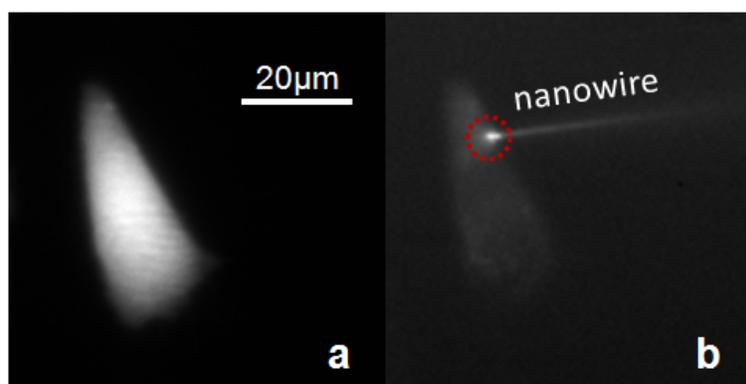
**Figure S12 Excitation of calcein AM stained HeLa cell through nanowire probe emission.** **a**, Fluorescence image of a live HeLa cell preloaded with calcein AM. Wide field illumination was used to excite the calcein fluorescence. **b**, Fluorescence/dark field image of the same HeLa cell being illuminated by the waveguided laser ( $\lambda=442$  nm) released from the tip of the nanowire probe showing a localized bright fluorescent spot, as marked by the dotted red circle.
