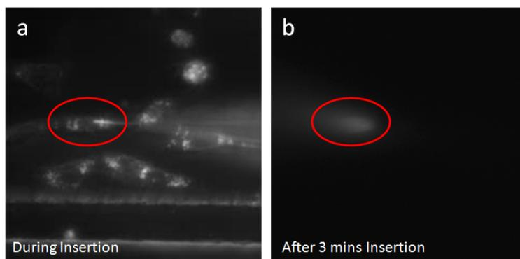
**Figure S10 Quantum dot (QD) delivery into a single living HeLa cell without irradiation.** **a**, Dark-field image showing the photoactivable QD-conjugated nanowire endoscope inserted into the cell. **b**, Dark-field image along with the excitation by the focused blue laser showing that no QDs were delivered into the cell after the insertion for 3 min without irradiation (photoactivation). 442 nm focused laser excitation and a 532 nm long-pass filter was used for the QD fluorescence imaging.
