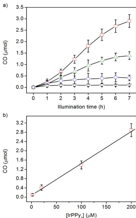
**Figure 7.** (a) Photocatalytic reduction of  $\text{CO}_2$  to CO in a 0.07 M TEA acetonitrile solution containing 0.2 μM **1c** and 0.2 mM (red squares), 0.1 mM (green triangles), 0.02 mM (blue circles), and 0.002 mM (black triangles)  $\text{Ir}(\text{ppy})_3$ , using a 130  $\text{mW}\cdot\text{cm}^{-2}$  Xe lamp fitted with an AM 1.5 filter. (b) Linear plot of CO production at the end of 7 h versus  $\text{Ir}(\text{ppy})_3$  concentration.
