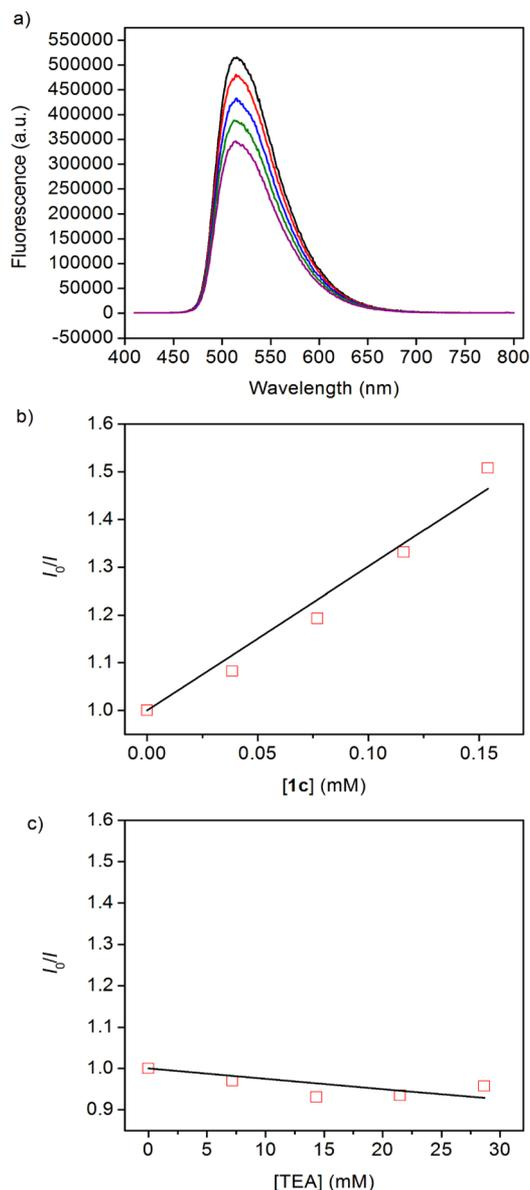
**Figure 8.** (a) Fluorescence spectra of an acetonitrile solution containing 0.05 mM  $\text{Ir}(\text{ppy})_3$  in the absence (black) and presence of 0.04 mM (red), 0.08 mM (blue), 0.12 mM (green), and 0.15 mM (purple) **1c**. (b) Linear plots of ratio of fluorescence intensities in the absence and presence of **1c** versus the concentration of (b) **1c** ( $y = 3021x + 1$ ,  $R^2 = 0.97$ ) and (c) TEA, according to the Stern–Volmer equation.
