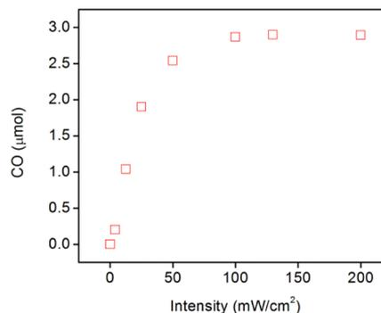
**Figure 6.** Photocatalytic reduction of CO<sub>2</sub> to CO in a 0.07 M TEA acetonitrile solution containing 0.2 mM Ir(ppy)<sub>3</sub> and 0.2 μM **1c** while varying the light intensity of a Xe lamp fitted with an AM 1.5 filter.
