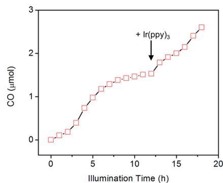
**Figure 9.** Photocatalytic reduction of CO<sub>2</sub> to CO in a 0.07 M TEA acetonitrile solution containing 0.2 μM **1c** and 0.2 mM Ir(ppy)<sub>3</sub>, using a 130 mW·cm<sup>-2</sup> Xe lamp fitted with an AM 1.5 filter. At 13 h, a fresh source of Ir(ppy)<sub>3</sub> was injected, and CO production was continued.
