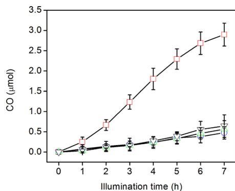
**Figure 5.** Photocatalytic reduction of CO<sub>2</sub> to CO in a 0.07 M TEA acetonitrile solution containing 0.2 mM Ir(ppy)<sub>3</sub> (black triangles), 0.2 μM **1c** (blue circles), 0.2 mM Ir(ppy)<sub>3</sub> and 0.2 μM Ni-(CH<sub>3</sub>CN)<sub>4</sub>(PF<sub>6</sub>)<sub>2</sub> (green triangles), and 0.2 mM Ir(ppy)<sub>3</sub> and 0.2 μM **1c** (red squares), using a 130 mW·cm<sup>-2</sup> Xe lamp fitted with an AM 1.5 filter.
