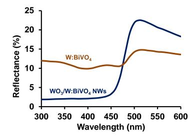
Figure S5. Reflectance of the  $WO_3/W:BiVO_4$  core/shell NWs and the 7 at%  $W:BiVO_4$  film (containing the same mass of Bi as coated onto the  $WO_3$  NWs).
