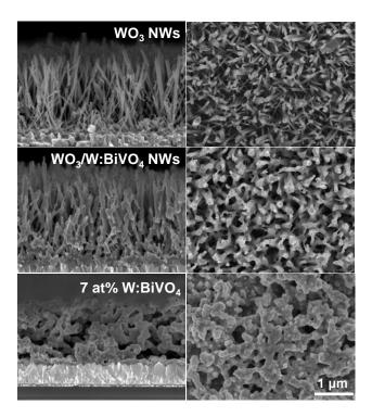
Figure S2. Scanning Electron Microscope (SEM) images of samples synthesized in this work. Left: side view, Right: top view of WO<sub>3</sub> nanowires (NWs), WO<sub>3</sub>/W:BiVO<sub>4</sub> core/shell NWs and 7 at% W:BiVO<sub>4</sub> film (containing the same mass of Bi as coated onto the WO<sub>3</sub> NWs). The scale bar applies to all images in the panel.
