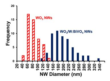
Figure S3. Histogram of diameters of the bare  $WO_3$  NWs and the  $WO_3/W:BiVO_4$  core/shell NWs. The bare  $WO_3$  NWs have a 75 nm average diameter and the average  $W:BiVO_4$  shell thickness is 60 nm.
