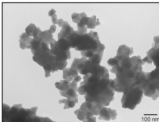
Fig. S4. TEM characterization of  $\alpha$ -NiS nanoparticles. TEM image of  $\alpha$ -NiS nanoparticles showing polydisperse hexagonal particles 20–100 nm in diameter.
