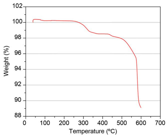
Fig. S5. TGA of  $\alpha$ -NiS catalyst. The absence of a significant loss in mass until  $\sim 450$  °C indicates a lack of surface-bound ligands on the  $\alpha$ -NiS nanoparticles. Experiment was performed under an atmosphere of  $N_2$  to prevent sample oxidation.
