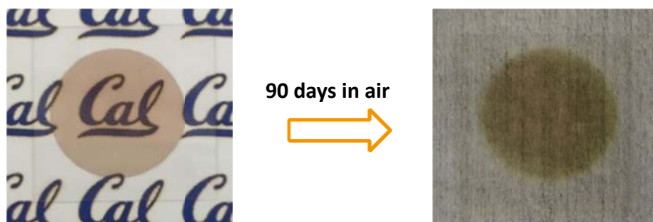
Figure S14. Copper film is fully oxidized after 3 months storage in air
